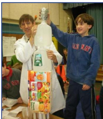
Testing the strength of paper columns.
